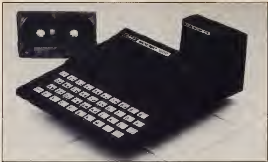
The TS 1000, with its buttonless "membrane" keyboard, sold 600,000 units in 1982. A more powerful version is coming this spring.
